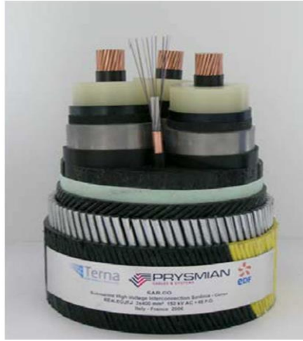
Figure 2.2: Sample of 132kV submarine cable (courtesy of Prysmian) (Source: FS report, July, 2024)
