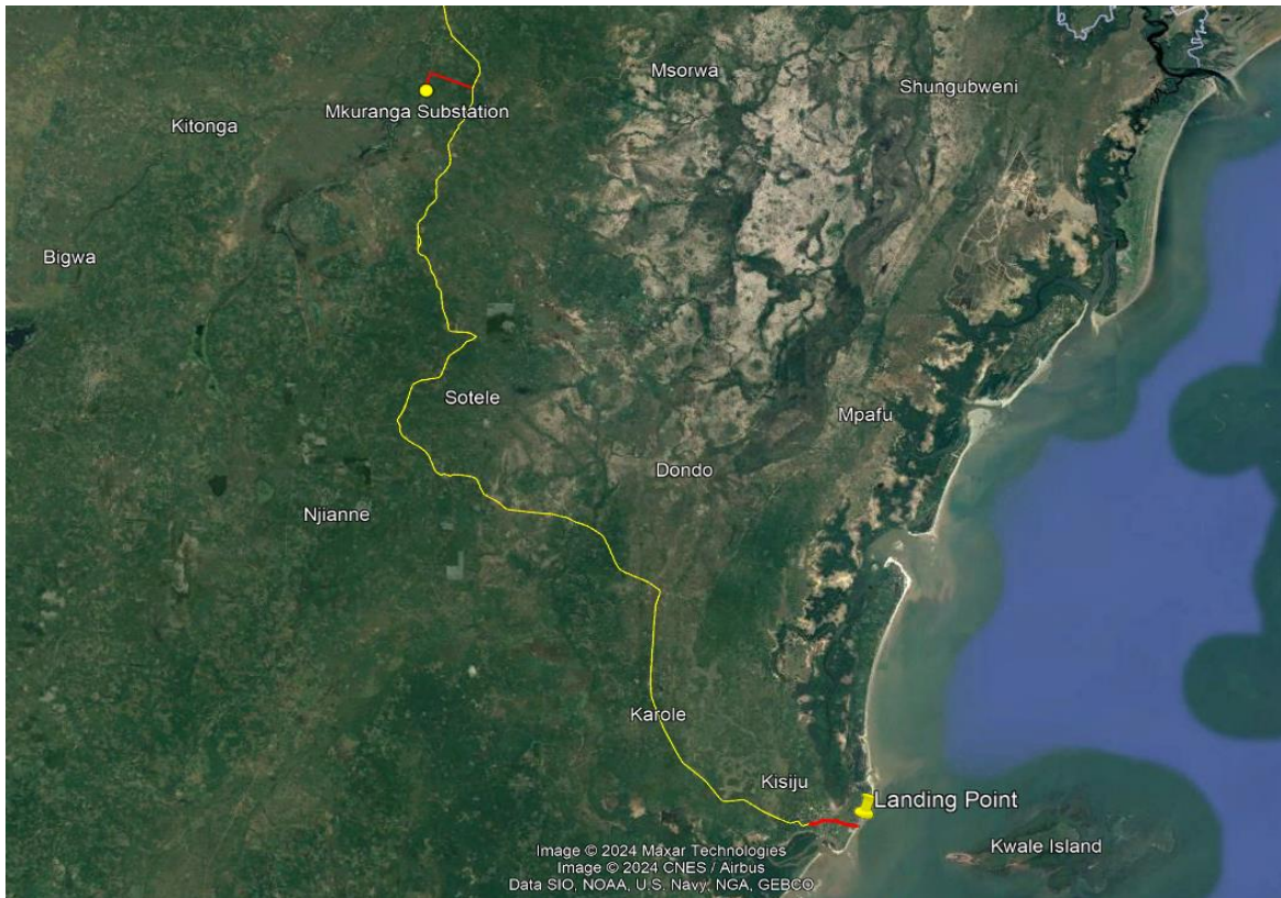
Figure 2:4: Map showing location of the transmission line route (0.5km - red line) from new Mkuranga substation, 35km Over Head Line (yellow line) and 2.5km underground cable (red line).
